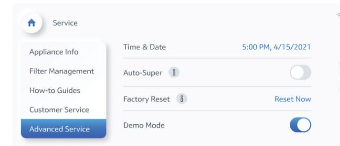
4. After enabling Demo Mode, the Demo Mode Home Screen will be displayed. After 3 minutes, the option to exit Demo Mode via the upper left button will no longer be displayed.
