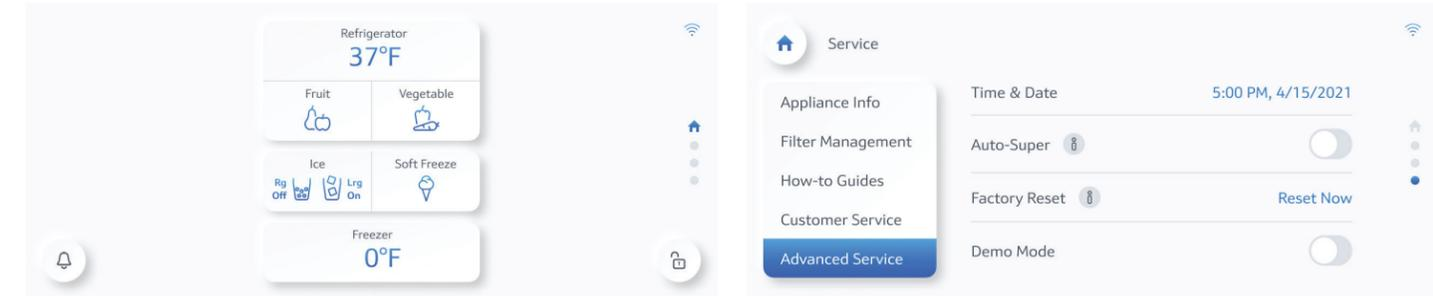
3. From the service menu, locate and tap on the Advanced Service section. Use the toggle next to Demo Mode to enable it.
