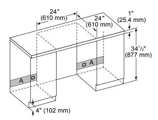
Recommended area for installation connection - a  $2^{1}/2^{"}$  (63 mm) diameter hole is recommended. Location of power cord at base of the appliance.
