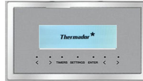
2. Use arrow keys on UI to scroll through the settings until Demo Mode Off option appears on the screen (right UI on double ovens).
