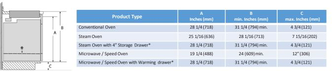
When installing an oven or oven with a drawer in combination with a cooktop, a minimum distance between the cabinet floor and countertop (B) is required. Reference the table for dimensions. Refer to the oven installation guide for all other measurements.
