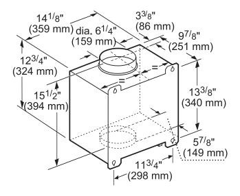
measurements in inches and mm
