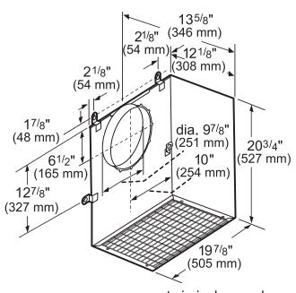
measurements in inches and mm
